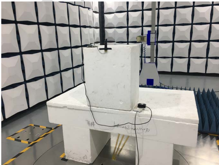
Radiated Spurious Emissions Test View (Above 1GHz)
